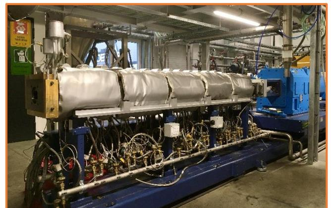
Twin screw extruder installation at JSW
